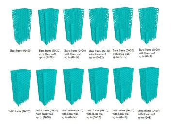
By using analysis methods like equivalent static lateral force method, response spectrum method and time history method analyzed these models to understand behavior of the structures from their results.
